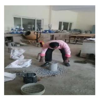
Bulk density test of coarse aggregate
